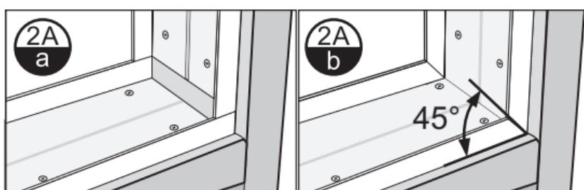
b. If mitering the ends, make all cuts at a 45° angle.
