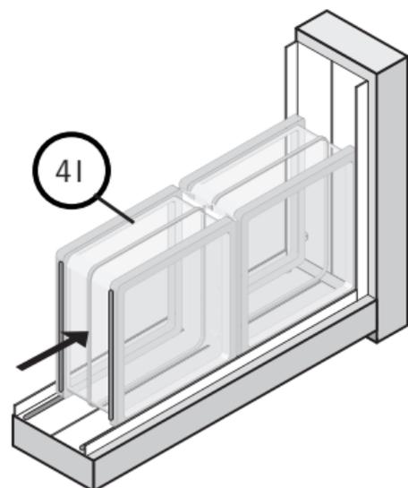
J. Continue inserting spacers and blocks in this manner to complete the row. Do not apply sealant to the side of the last block and last spacer. Insert the last block in the side channel and slide it into the bottom channel.
