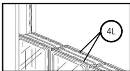
M. Place a horizontal spacer on top of the first row of blocks. If more than one section of horizontal spacer is required, be sure to lay them end to end with the joint directly above vertical spacer. Stagger these joints on each following row.
