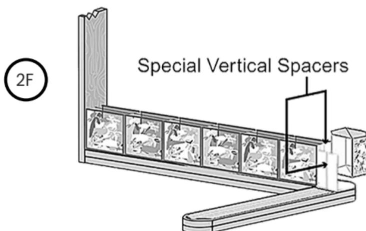
G. The vertical spacers for AllBend™ blocks are tapered, the spacers for 90° blocks are flat. The smaller end is placed at the back of the AllBend™ block. The appropriate vertical spacers are packaged with the shaped horizontal spacers. Tridron® and sharp 90° corners and EndBlock™ are standard vertical spacers.
