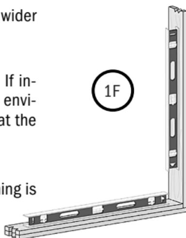
G. Verify all measurements. Remember, for rough opening's total height, add 1/4" to width measurement
