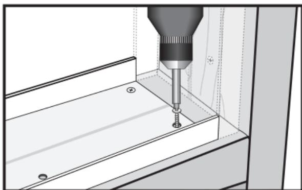
*Note: If the pre-drilled holes at the ends were trimmed off when cutting the channel to length, drill new ones at the ends of the cut piece.*
