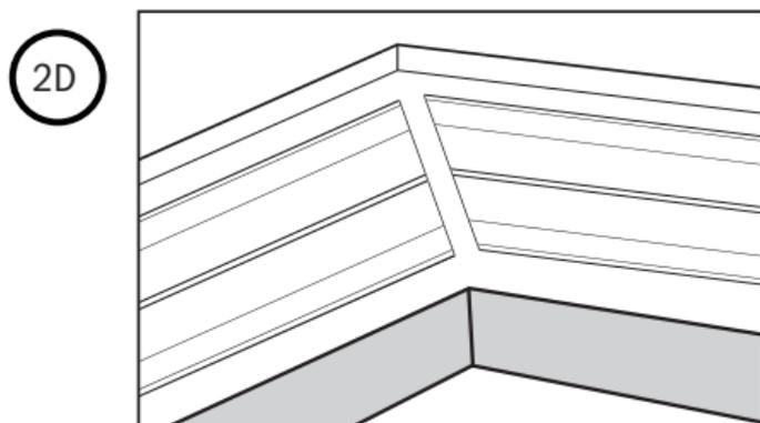
E. Install the first row of blocks and vertical spacers, starting with first block in the jamb.
