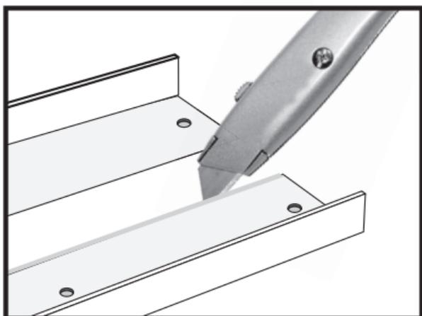
*Note: Cutting the top channel in half will allow the top row of blocks to be installed. If panel is only one or two blocks wide, side channel will also need to be cut in half.*
