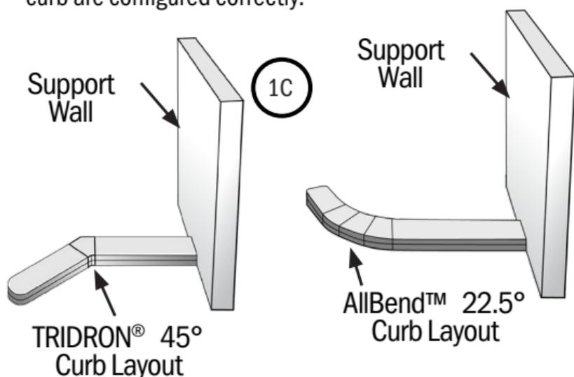
D. The curb must be as wide as, or wider than, the glass block thickness.
