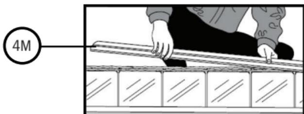
N. Remove any excess sealant. If necessary, adjust the size of the sealant beads to prevent squeeze out on the following rows. The joint areas must be kept clean of sealant.
