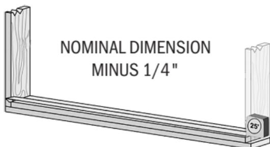
*Note: If it is necessary to have a joint in the horizontal spacer, to extend it to fit the width of the section, make sure the joint will align with a vertical spacer. Stagger these joints on each following row.*
