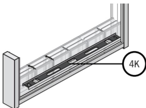
L. Apply two 1/4" beads of sealant to the top of the row of blocks just behind the raised edges.
