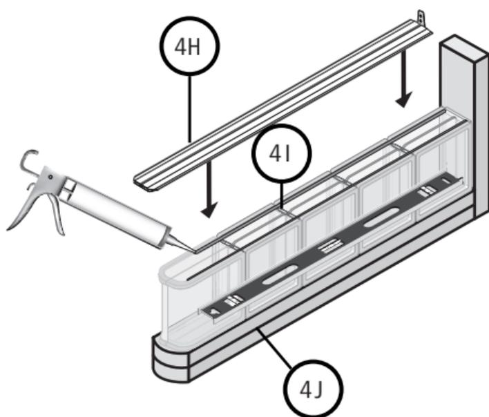
I. Remove any excess sealant. If necessary, adjust the size of the sealant beads to prevent squeeze out on the following rows. The joint areas must be kept clean of sealant.
