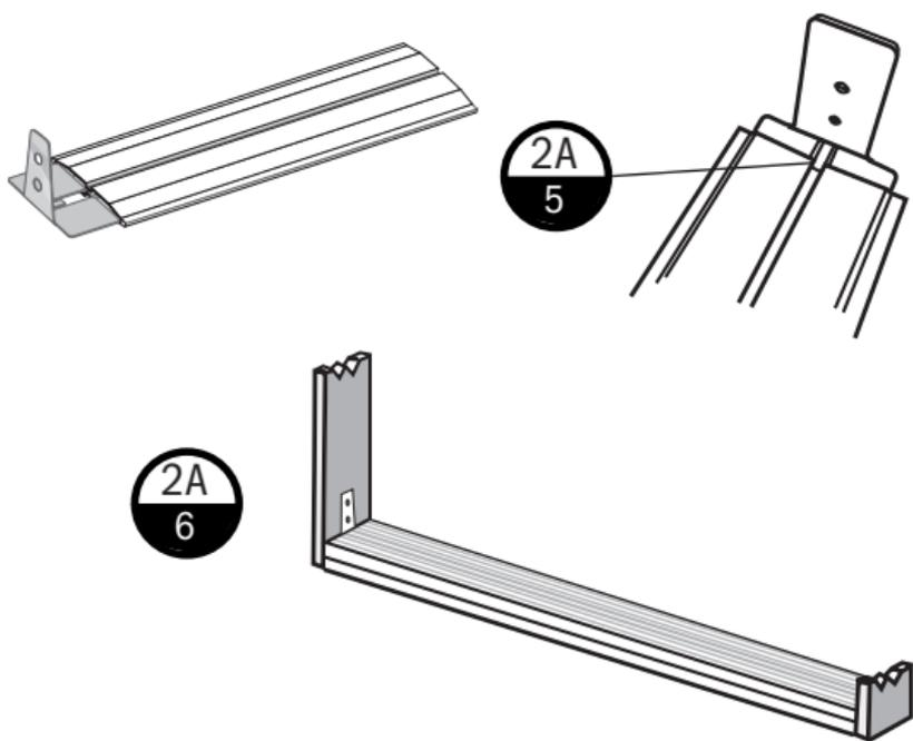
6. Place the spacer in the bottom of the opening, centered in the section. DO NOT install with screws.
