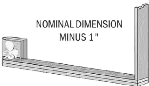
3. For straight sections between a shaped block\* and an EndBlock™, cut the horizontal spacer  $3/4"$  shorter than the nominal dimension.
