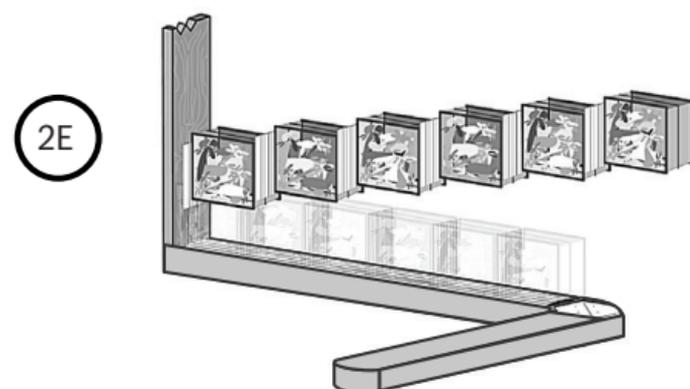
F. There are special vertical spacers for shaped blocks. Be sure to insert these spacers before, between and after shaped blocks.
