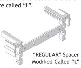
• Where glass block meet the jambs and curb, (except for the four corners) orient the spacer with the cross arm down and clip off the upper set of toothed legs, and the upper half of the twist-off tab.
