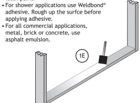
If using Weldbond®, apply mortar to the surface before it cures. Otherwise, let the treated area set up and cure before installing the first row of block.
