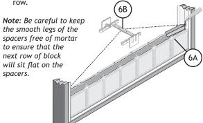
B. Place a "FLAT" spacer on top of the first and last block of the previous row where they meet the side channels. C. Set the first block and last block of the next row into the side channels on top of the "FLAT" spacers.
