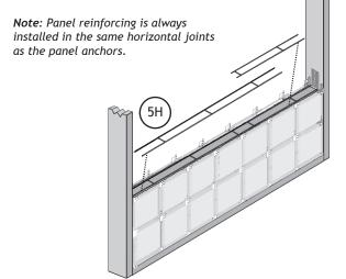
**Note:** If using 12" x 12" nominal size glass block, panel anchors and panel reinforcement should be installed on top of every row, except the top row.
