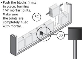
D. Remove excess mortar with a polyfoam brush, and fill any voids on both sides of the panel.
