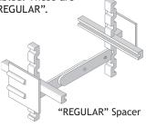
• For the two bottom corners of the panel, orient the spacer with the cross arm down and clip off the upper toothed legs. Clip off the upper half of the twist-off tabs. Cut off the left or right side of the remaining twist-off tab and the smooth legs on the same side. Only two of these spacers are required. Clip off the right set of smooth legs of one spacer, the left set of the other spacer. These are called "L".
